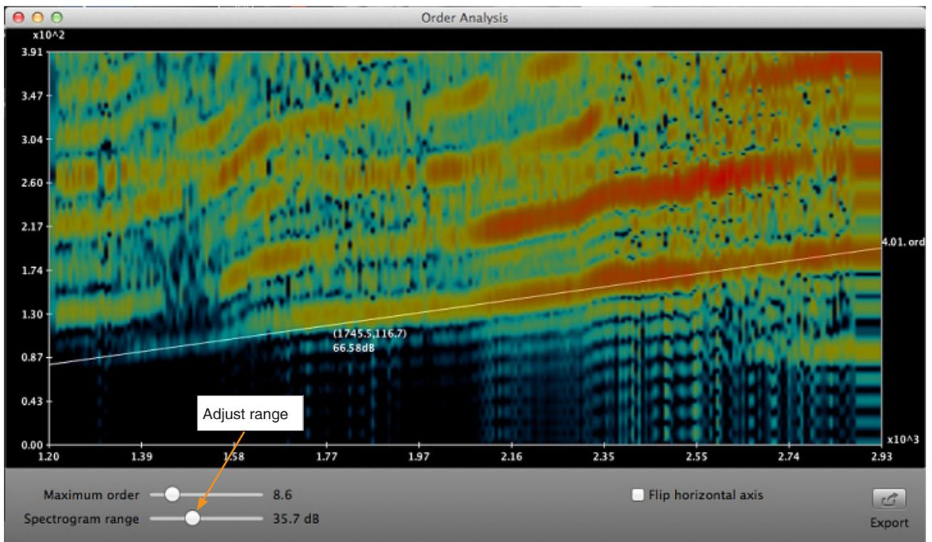
By pressing the spectrogram label on the lower left it is possible to see the values for the straight line going through the spectrogram.
