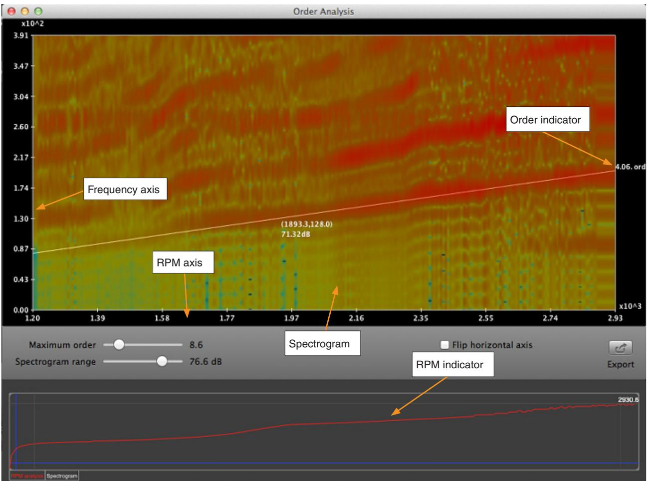
There are two adjustments for the spectrogram, either the maximum order in the spectrogram, or the dynamic range, can be adjusted
