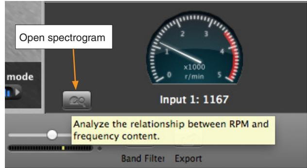
The order analysis window will pop up with the spectrogram on the top and an RPM indicator on the bottom. The grey lines in the RPM indicator are chosen automatically to select a section of constant increasing (or decreasing) RPM, which the analysis is composed of. In the spectrogram window, frequency as a function of RPM is plotted. By moving the mouse cursor inside the spectrogram window, it is possible to read off the order indicator on the right side of the screen.
