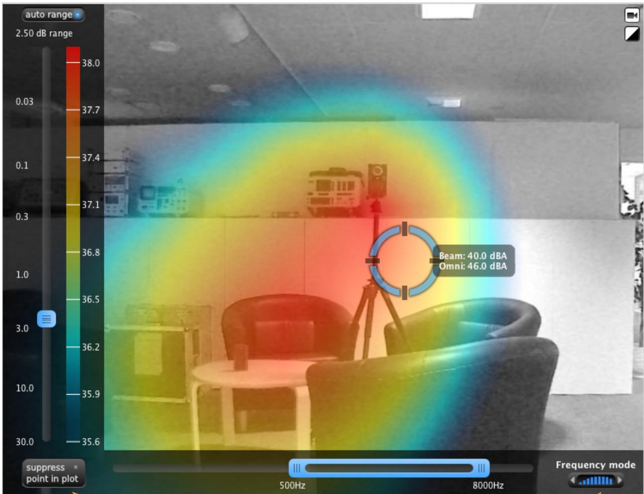
The acoustic eraser is enabled by pressing the suppress point in plot button
