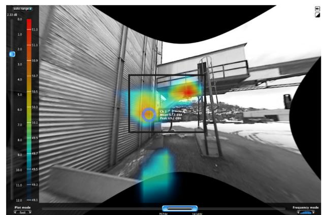
**By zooming in, a higher resolution is obtained for the interesting part of the picture** The next picture shows the display after the zooming operation. A grid is placed on the picture to show the acoustic resolution for the level colouring (Frequency band).
