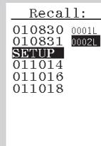
To display the files contained in the selected folder, press the **▶** key and locate the file in question by means of the vertical cursor keys.
