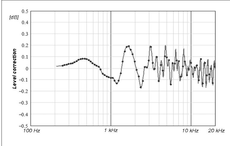
Case reflections for Nor 131 for sound approaching the microphone from the front along the axis of symmetry. The diagram shows the level difference between the response for the microphone-preamplifier alone (extension cable) and when mounted on the instrument
