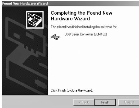
6. The installation of the USB driver is complete when this picture appears.
