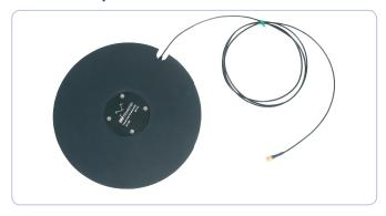
This triaxial seat accelerometer is designed for whole body measurements according to ISO2631 and ISO8041. The integral cable is 2m and the connector fits the Nor133 and Nor136 vibration meters. The seat pad consists of a rubber pad, an aluminum mounting adapter plate to where a triaxial accelerometer type Nor1288 is mounted. The Nor1288 accelerometer port is detachable for calibration purpose.
