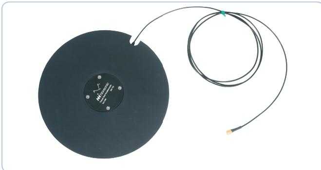
This triaxial seat accelerometer is designed for whole body measurements according to ISO2631 and ISO8041. The integral cable is 2m and the connector fits the Nor133 and Nor136 vibration meters. The seat pad consists of a rubber pad, an aluminum mounting adapter plate to where a triaxial accelerometer type Nor1288 is mounted. The Nor1288 accelerometer port is detachable for calibration purpose.
