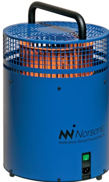
The reference sound source Nor278 is designed to produce a stable and uniform sound power output with unique long-term stability. The high sound power output makes it ideal for sound power measurements in a noisy environment. The rugged, but yet portable and light weight construction is perfect for field use as well a laboratory use. Every effort is made in the design to ensure a uniform frequency response and optimum directional characteristic well inside the requirements in ISO 6926.
