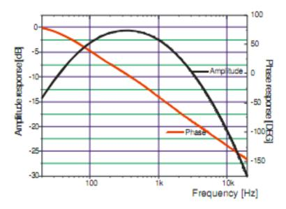
Figure 3. Velocity response model
