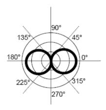
Figure 4: Particle velocity sensor polar pattern
