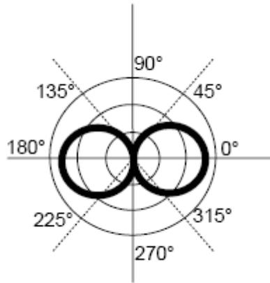
Figure 4: Particle velocity sensor polar pattern
